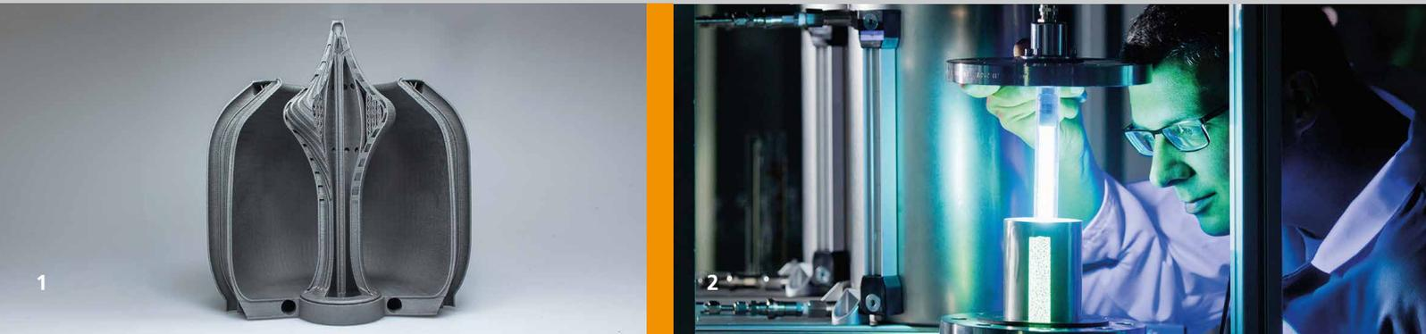
**1** Rocket propulsion with aerospire nozzle made of high-temperature resistant alloys for future space applications. Manufactured using Selective Laser Melting SLM, the engine features complex, conventionally non-producible cooling structures capable of withstanding temperatures in excess of 2000 Kelvin (© Fraunhofer IWS).
